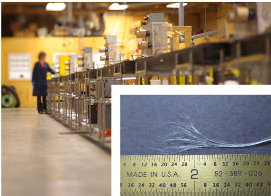
Figure 1: (a) (below) bench scale solution spinline, (b) (right) air gap (dry-jet) wet spinning, (c) (bottom right) multifilament, continuous polyacrylonitrile (PAN) precursor tow, and (d) (bottom center) close up of multifilament precursor tow
