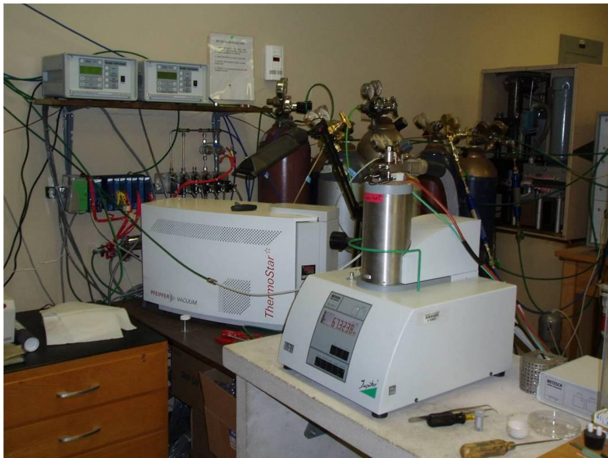
TG/DTA/MS with gas controls for blending and switching gases for oxidation/reduction cycling
