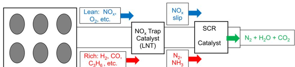
Fig.1 Coupled LNT-SCR System for NO<sub>x</sub> reduction
