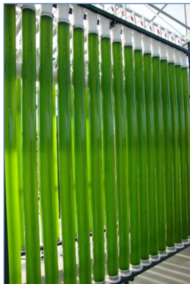
Figure 1 (Left). 1000 L Tubular Photobioreactor
