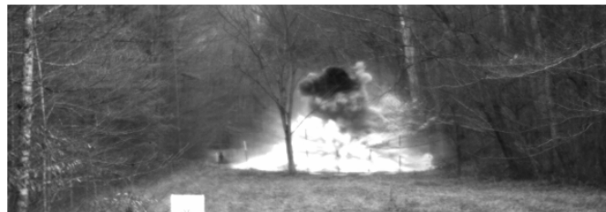
Explosion cloud from 200-lb charges 10-ms after detonation: 20% coated AN (top); 100% ANFO (bottom).
