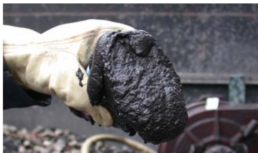
Paste-thickened material obtained from a pilot-scale test
