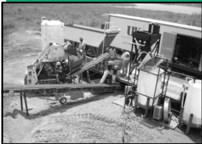
CAER researchers 'scalping' the feed samples at the LG & E plant in Ghent, Kentucky.
