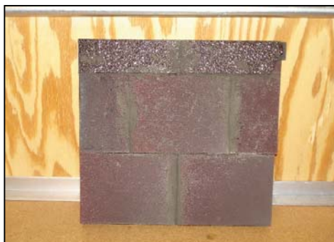
A sample of 6" square roofing tile made from Koppers L-foam, coated with a commercial ceramic glaze.
